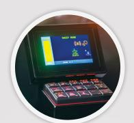
controls: Bright state-of-the art HUD with sealed tactile control pad optimized for ease of use. 360° flexible RAM MOUNT location adjustment allows
