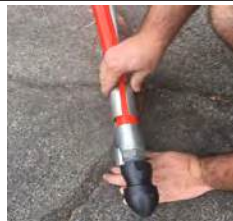
1) Place hose in jaws 2) Close Jaws around hose 3) Lower the guide into place 4) Pull rope and release hose and nozzle
