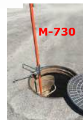
1) Place hose in jaws 2) Close Jaws around hose 3) Lower the guide into place 4) Pull rope and release hose and nozzle
